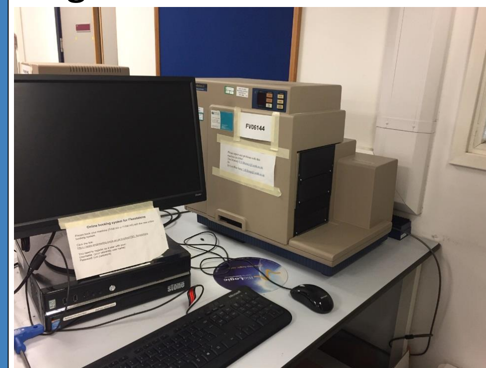
Figure 2: A Flexstation emits a laser at 340nm and 380nm to excite the Fura-2 stain, which when bound to calcium will absorb more light energy at 340nm compared to 380nm and hence fluoresce more strongly. This creates an excitation ratio (F340/F380) which can be used to quantify the intracellular calcium load.
