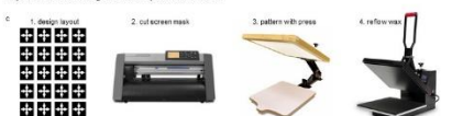
Figure 4. (A) Carnauba wax patterning showing the formation of a solid hydrophobic barrier in a two-step application. (B) An initial attempt to quantify the resolution of the patterning process. (C) Workflow for patterning paper using a non-traditional screen printing approach.
