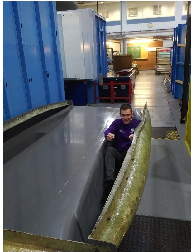
Fig. 5. The completed chassis mould, ready for lay up.
