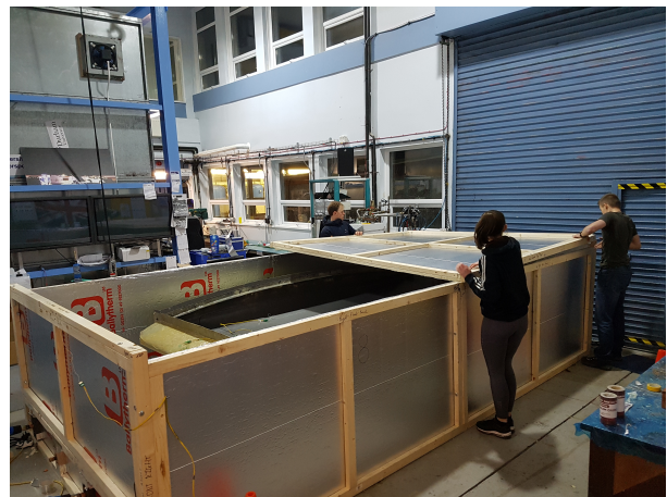
Fig. 3. The mould in the 5m oven ready for post cure.
