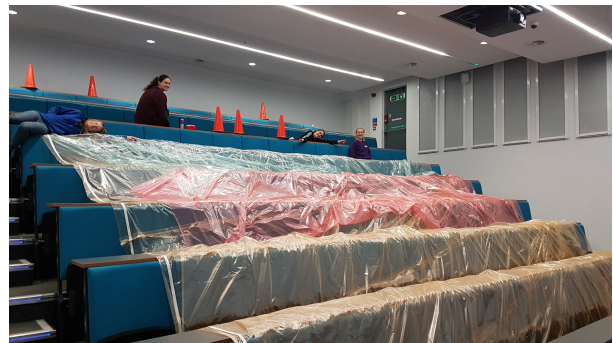
Fig. 6. The very large vacuum bag used to cure the aerostructure.
