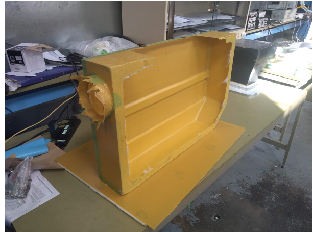
Fig. 9. The battery box immediately after being released from the mould but before being trimmed and having holes for bolting components put in.
