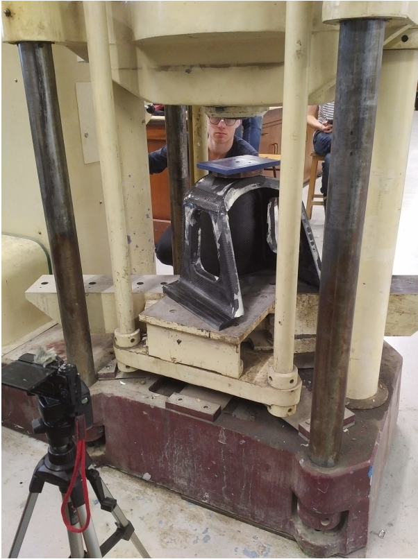
Fig. 4. The test roll-hoop undergoing a compression test to verify correlation between computational analysis and physical strength.
