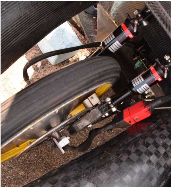
Fig. 8. The rear motor side suspension, showing the carbon fibre trailing arm and the bicycle air shocks.
