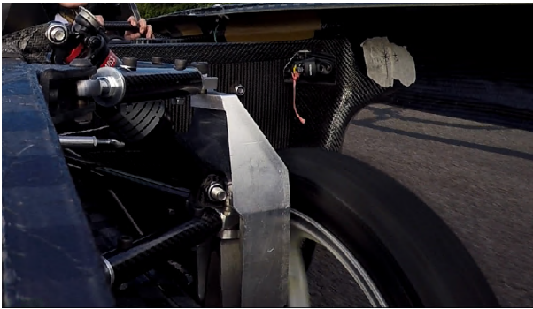
Fig. 7. The front suspension showing the carbon wishbones, aluminium upright and bicycle shock.
