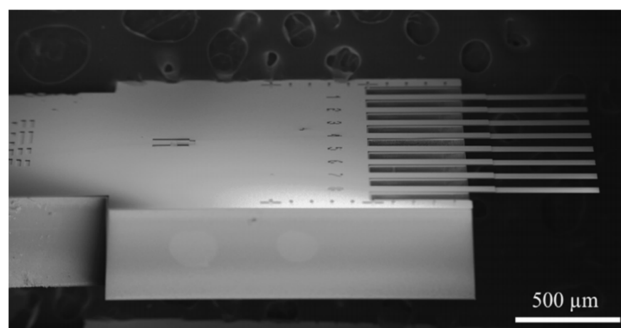
Figure 2: A typical cantilever array 3 .
