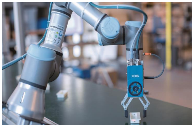
Figure 13. SICK sensor mounted directly next to the end effector. (Mead, 2019)
