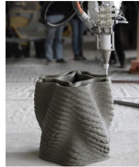
Figure 8. An end effector designed and refined to 3D print with a specific mixture of clay (Anton, et al., 2020, p. 291)
