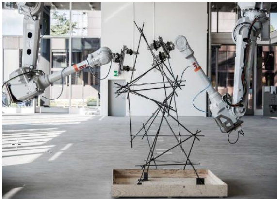
Figure 16 degree of freedom robots assembling a structure from steel (Parascho, et al., 2020, p. 27)
