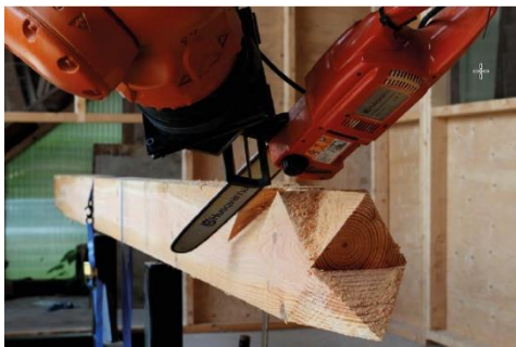
Figure 9. The use of commercially available chainsaws with triggers zip-tied in place. (Self & Vercruyssen, 2020, p. 33)
