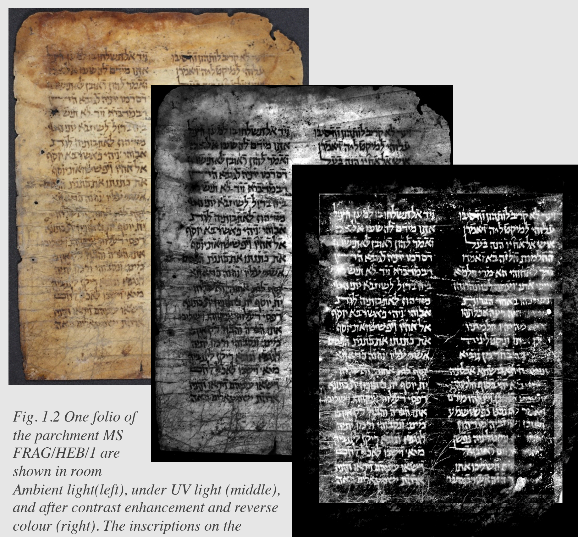
Fig. 1.2 One folio of the parchment MS FRAG/HEB/1 are shown in room Ambient light (left), under UV light (middle), and after contrast enhancement and reverse colour (right). The inscriptions on the parchment are getting more and more Readable with more processing on the images are taken. This case shows the possibility of applying other image processing techniques for the same results to make the content more distinguishable. Part of the inscriptions are further enhanced to see its contour (right).
