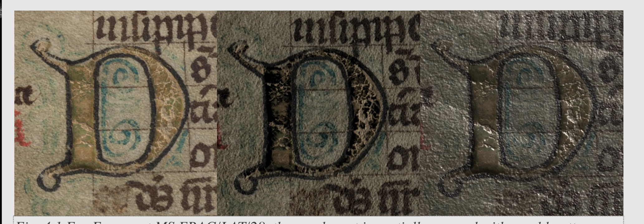
Fig. 4.1 For Fragment MS FRAG/LAT/28, the parchment is partially covered with a gold pattern as shown in the graph above, to determine the details of its corrosion for conservational purpose, RTI is carried out (middle) and specular enhancement is also processed for a more precise look of the surface structure (right).
