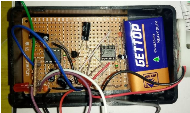
Figure 12 - The circuit simulated inside the box
