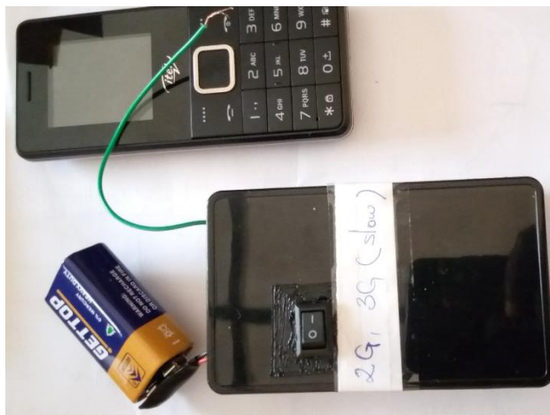
Figure 13 - Cell phone detector enclosed (device) with cell phone aside
