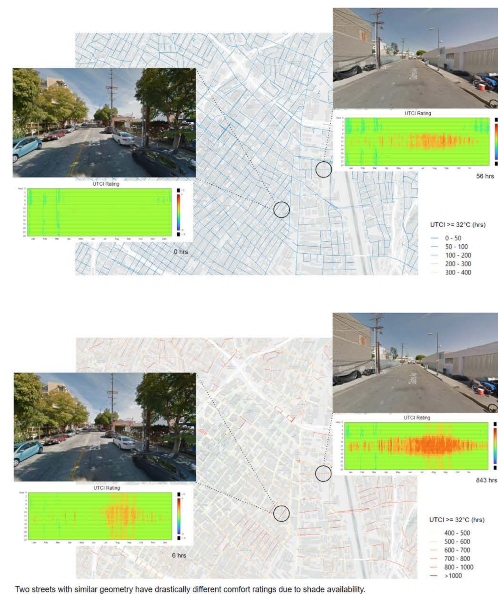
Two streets with similar geometry have drastically different comfort ratings due to shade availability.
