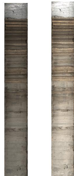
Figure 1. Images of the Baltic Sea sediment core, section 4, taken from the XRF scanner. (Authors own)
