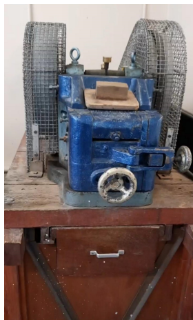
(a) Jaw crusher Used to Break Gneiss Samples.
