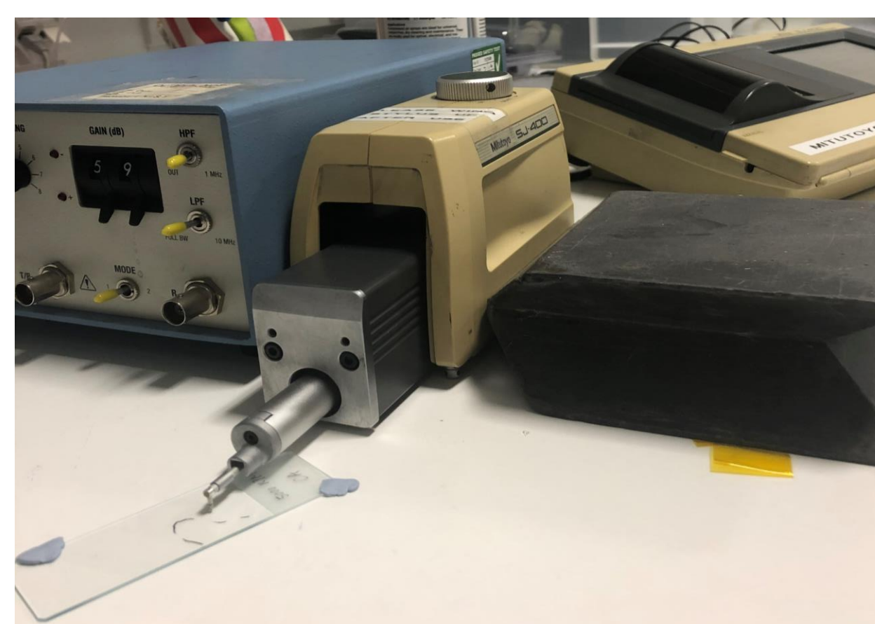
Figure 6: A contact profilometer which measures the thickness of the layers CA, PVK and PMMA
