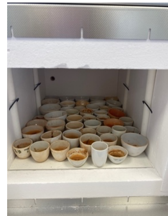
Diagram 6: A collection of soil samples in the furnace
