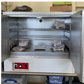
Diagram 3: Oven used to dry samples
