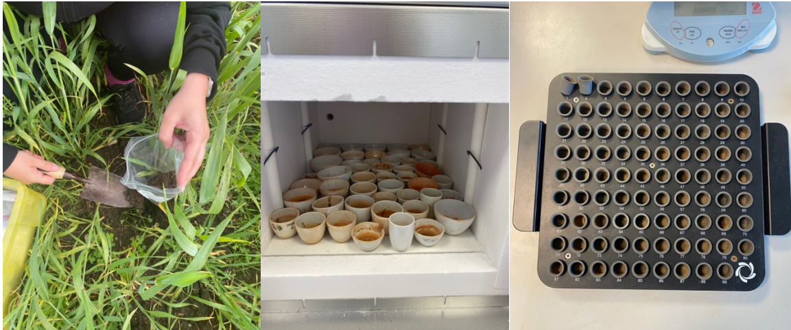
Figure 1: A photo of soil sampling in the field. Figure 2: A photo of crucible samples in the furnace. Figure 3: A photo of the Elementar soliTOC Cube sample tray.
