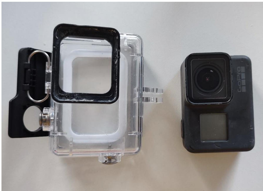
Figure 9: GoPro camera and its protective case. Notice that the lens protector was removed after it was cracked.
