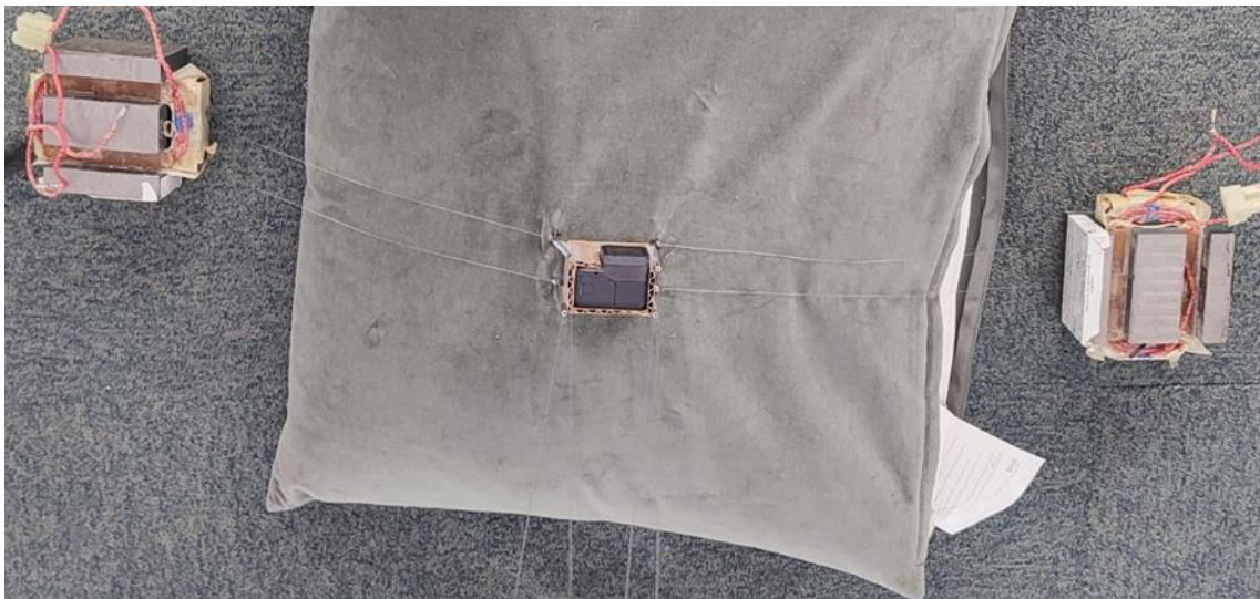
Figure 23: Second string-rail prototype. Top view of the camera in the holder on top of the pillow.
