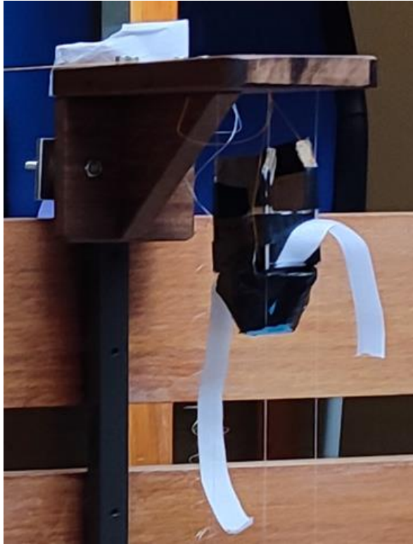
Figure 8: Camera holder with the safety Velcro strap and the aerodynamic tip.
