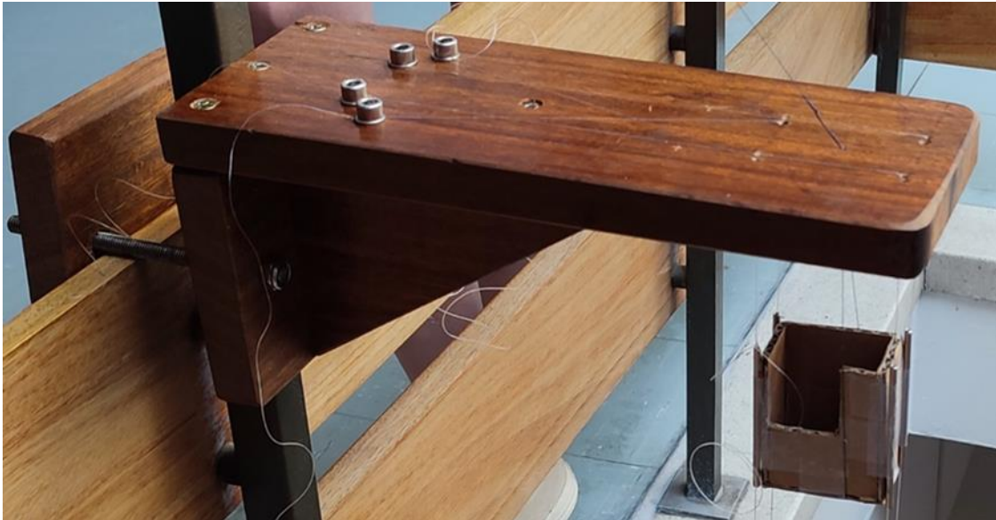
Figure 10: The drop platform fixed to the handrail of the second floor at the School of Physics. The holder in the picture is not the final design produced.
