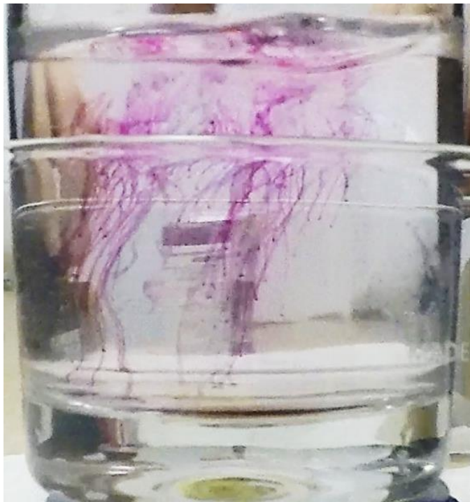
Figure 7: Potassium permanganate dissolving in a glass of water that has been recently spun retaining angular momentum. The picture has been edited to make the purple traces more noticeable
