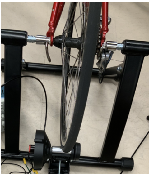
Fig. 4: Brushless DC, RC Motor Connected to the Bicycle Trainer for Power Generation
