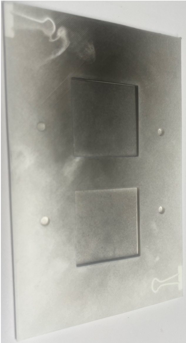
Figure 3: The acrylic mask with the deposited carbon black solution on the cardstock.
