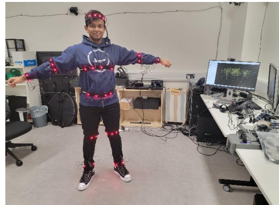
Figure 23: Me (Author) rigged with the PhaseSpace LED lights (Whole body)
