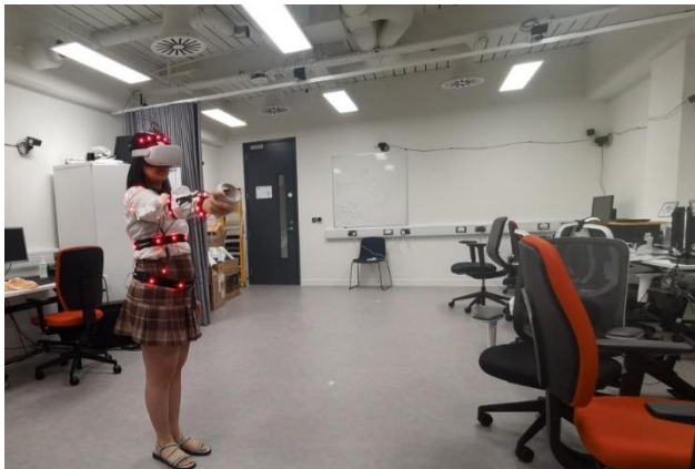
Figure 22: A human rigged with the PhaseSpace LED lights (Upper body only)
