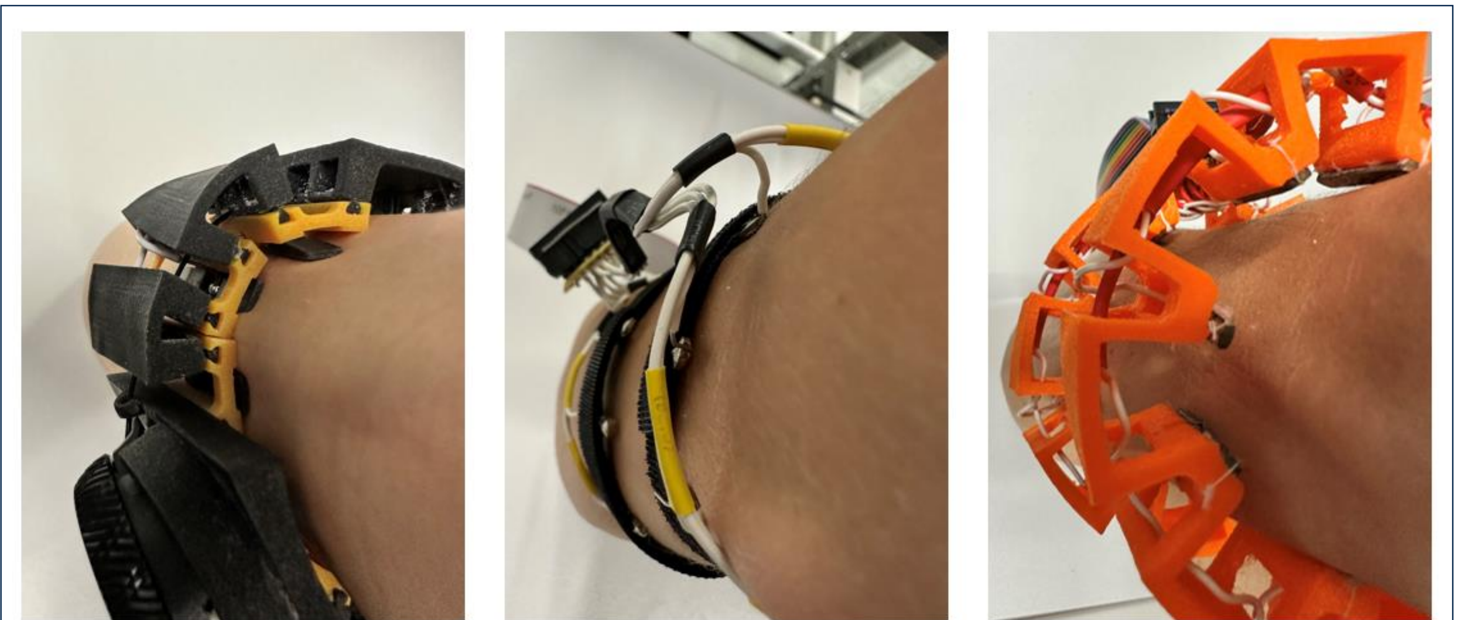
Figure 5: Comparison of fit tightness between new design (left) and old designs (middle and right)
