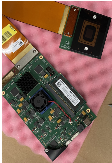
Figure 2: The DMD with the corresponding electronic board
