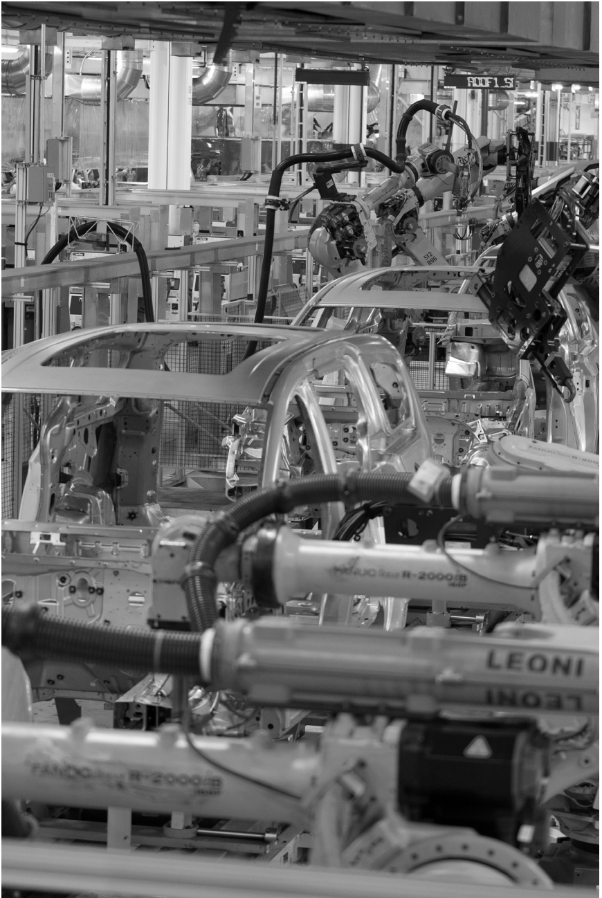
Robotic arms have completed most of the welding at the Chrysler Assembly Plant since their addition in 1983 / Stellantis Media North America
