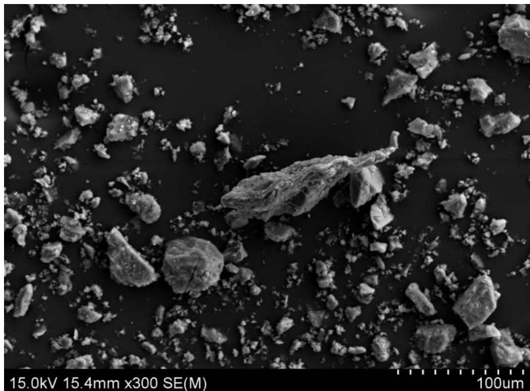
Figure 17. Smaller crystal structures in WWTP struvite samples
