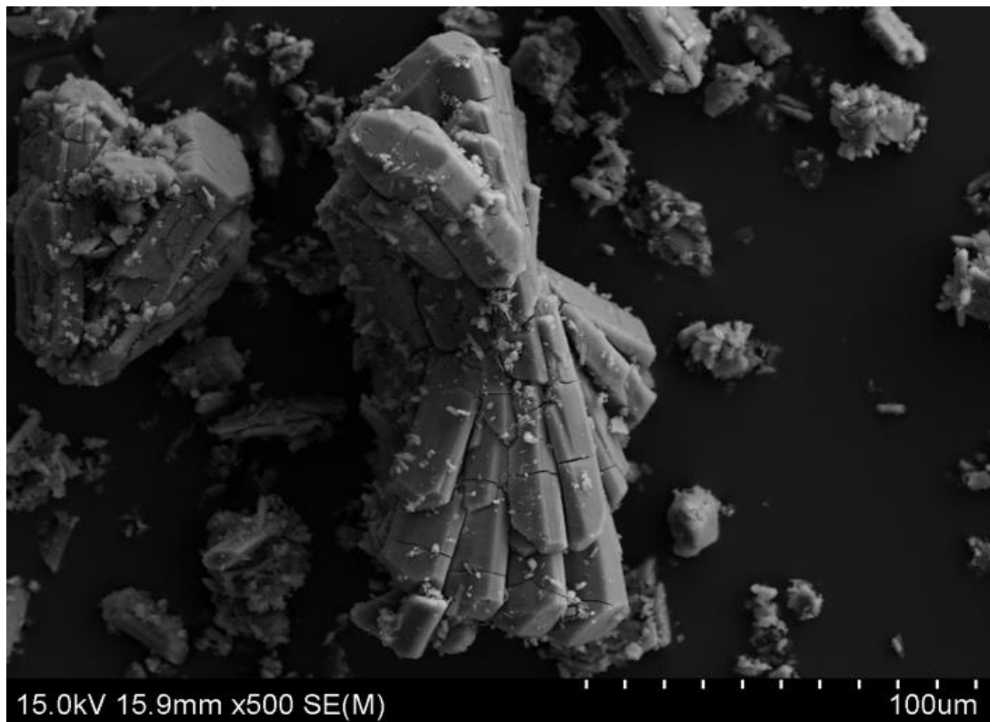
Figure 12. SEM image of carbonated synthetic struvite
