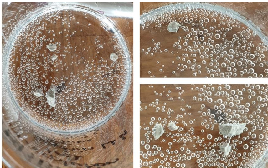
Figure 26. Nucleation Sites on the chunks of WWTP struvite when submerged in carbonic acid
