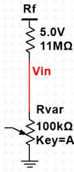
Fig. 3. Voltage divider circuit for calculating realtime resistance of the FSR and hence deducing the applied contact force.
