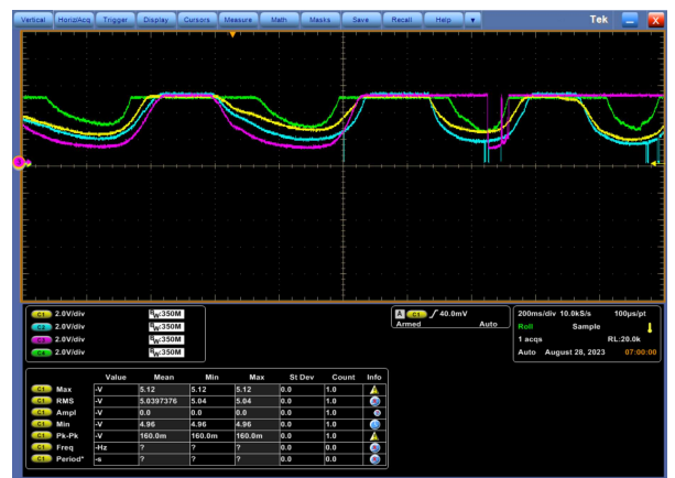
Fig. 7. Oscilloscope readings of the FSR response to touch stimulus from the human hand.
