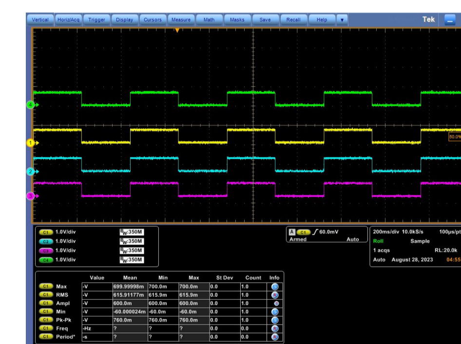
Figure 5: Oscilloscope reading of the buffer output and original signal input (blue:original input signal, other colors: buffered output).
