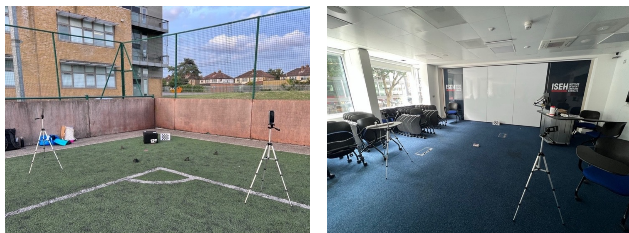
Figure 1. Left: Outdoors set-up at the football field during a data collection session in July; Right: Indoors set-up at the Institute of Sports Health and Exercise during testing OpenCap
