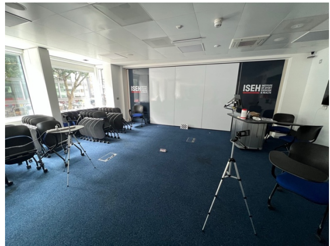
Figure 1. Set-up for data collection with OpenCap using two smartphones
