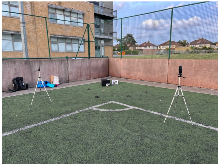
On-site set-up showing the whole capture volume and calibration checkerboard. Photo taken on 11 July 2023 (Tuesday)
