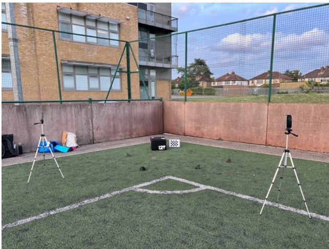
Figure 1. Set-up for data collection with OpenCap using two smartphones
