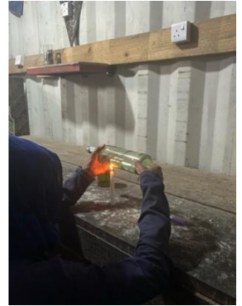
Step 4: Put fire over engraving and rotate, then blow into bottle, causing it to separate into two parts
