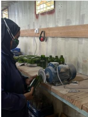
Step 5: Use sanding disc to smooth out edges and top of glass.
