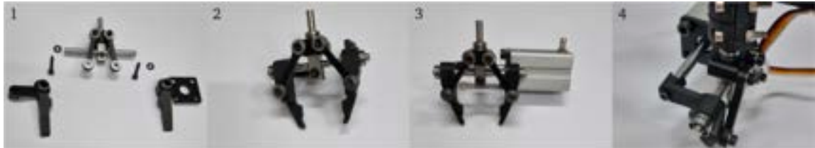
Fig. 14. Gripper in disassembled state (1). Slide the selected gripper fingers (gripping surfaces pointing inwards) onto the horizontal linear guide rail via the linear bearings and screw the gripper fingers to the movable holders (2). Attach the gripper to the pneumatic cylinder and cylinder rod via the screw connection points (3). Attachment of the entire gripper to the robot via the muff coupling (4).
