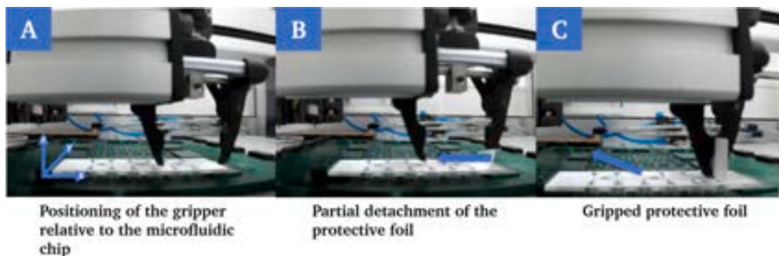
Fig. 19. After the parallel gripper has been positioned centrally relative to the chip at the cut-out height so that it opens and closes along the negative x-axis (A), partial removal of the protective foil begins by closing the gripper (B). The robot then moves along the negative x-axis and, from the last third of the chip length, also performs a movement in the positive z-direction until the foil is completely removed (C).
