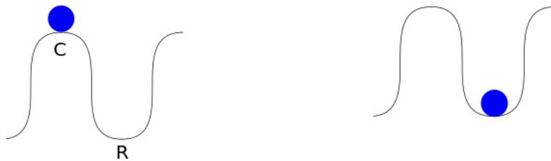
Figure 6: Schematic of a ball going down to a valley to minimize its energy
