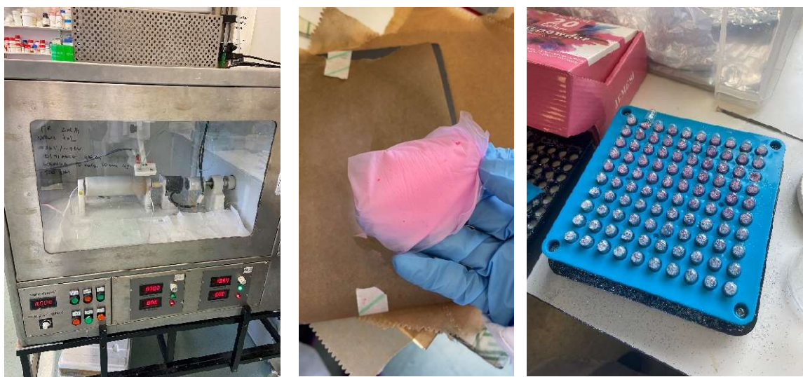
Images of the electrospinning equipment (left) used to create colourful orodispersible films (middle), and using a capsule press to make sucrose/glitter capsules (right)
