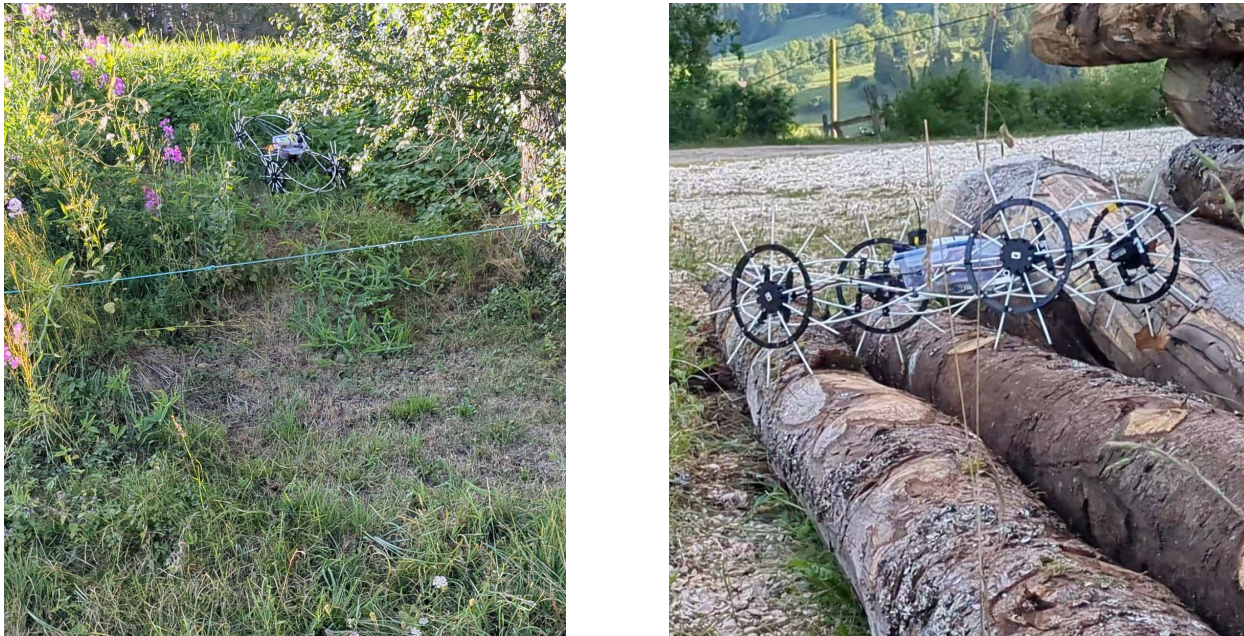
Figure 11: Overcoming 45° slopes and logs
