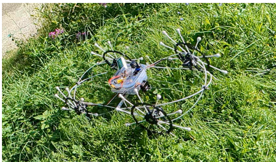
Figure 9: PLA ends mounted on top of the spokes
