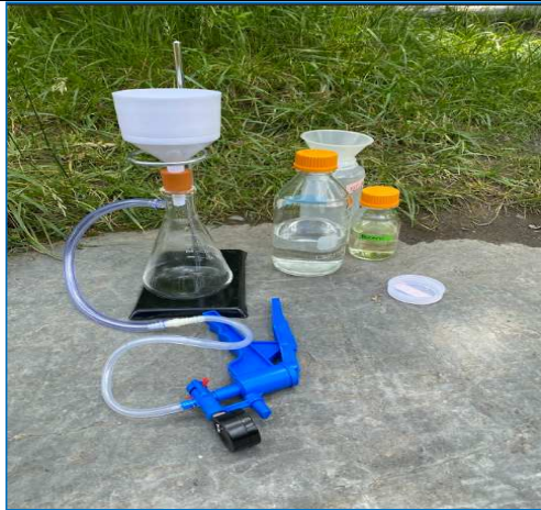
Figure C, set up of the sampling station on the field site. Figure D shows sampling station in lab. The filter paper goes in the Büchner funnel (the white funnel), water sample is poured down the funnel and the blue hand pump is used to create vacuum in the flask that will draw the water through the filter.
