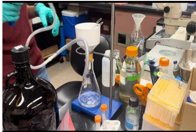
Figure C, set up of the sampling station on the field site. Figure D shows sampling station in lab. The filter paper goes in the Büchner funnel (the white funnel), water sample is poured down the funnel and the blue hand pump is used to create vacuum in the flask that will draw the water through the filter.
