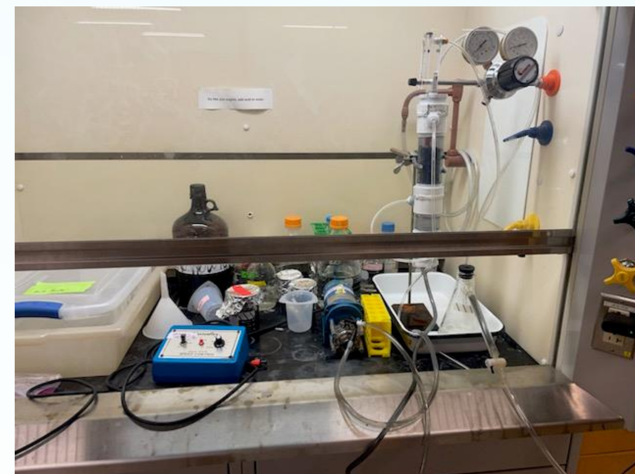
Image of ammonia volatilization reactor set up in fume hood.
