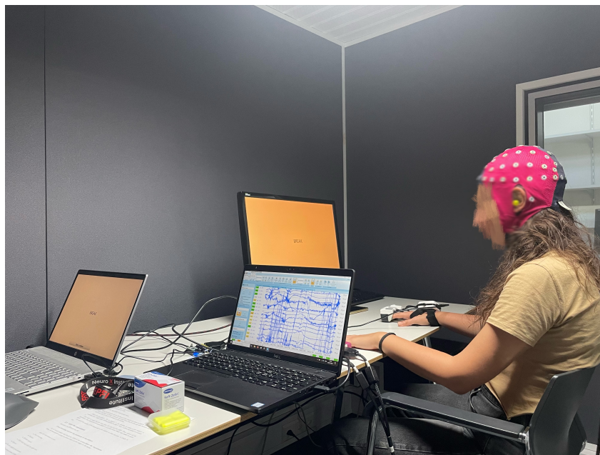
Figure 1: A participant undergoing EEG data acquisition while responding to tactile stimuli. The participant wears a 64-channel EEG cap, and real-time data is captured on the connected monitor. The experimental setup includes multiple screens for stimuli presentation and EEG signal monitoring.
