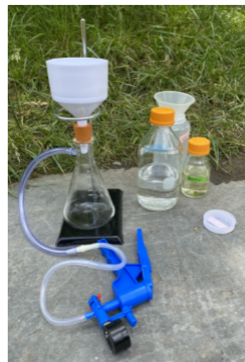
Figure 2. Active filtration apparatus using a hand pump.
