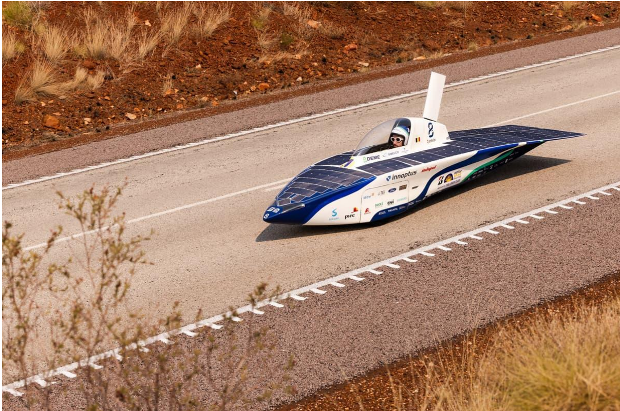
Figure 4: An example of the proposed canopy fin geometry as seen on the 2023 Innoptus solar car [9]
