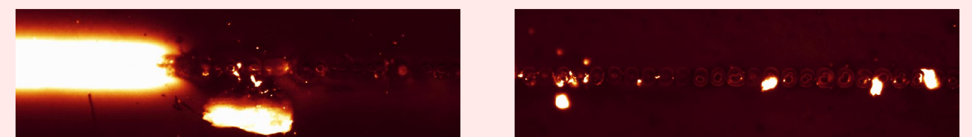
Rhodamine B dyed glass mold with PDMS residues under a fluorescence microscope
