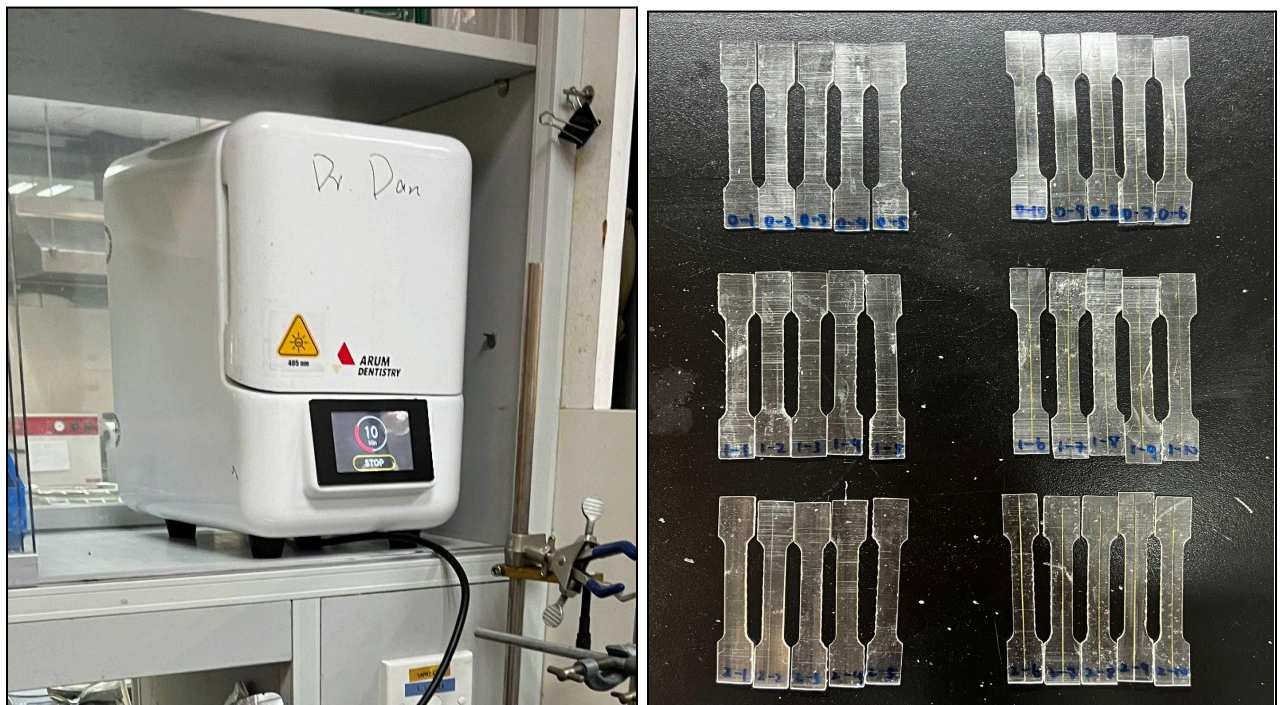
UV Curing Chamber (Left) and Completed Specimen Display (Right)
