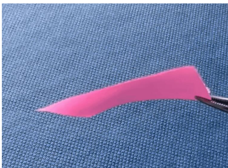
Figure 1: A thin polymeric film consisting of a polymer solution combined with rhodamine (an artificial dye).
