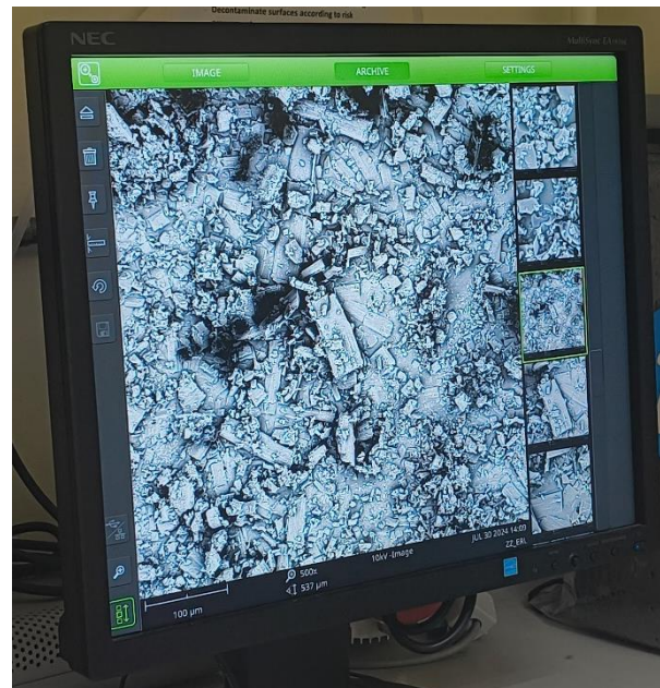
Figure 5: A scanning electron microscopy (SEM) image of amorphous structure found in a prototype ODF.
