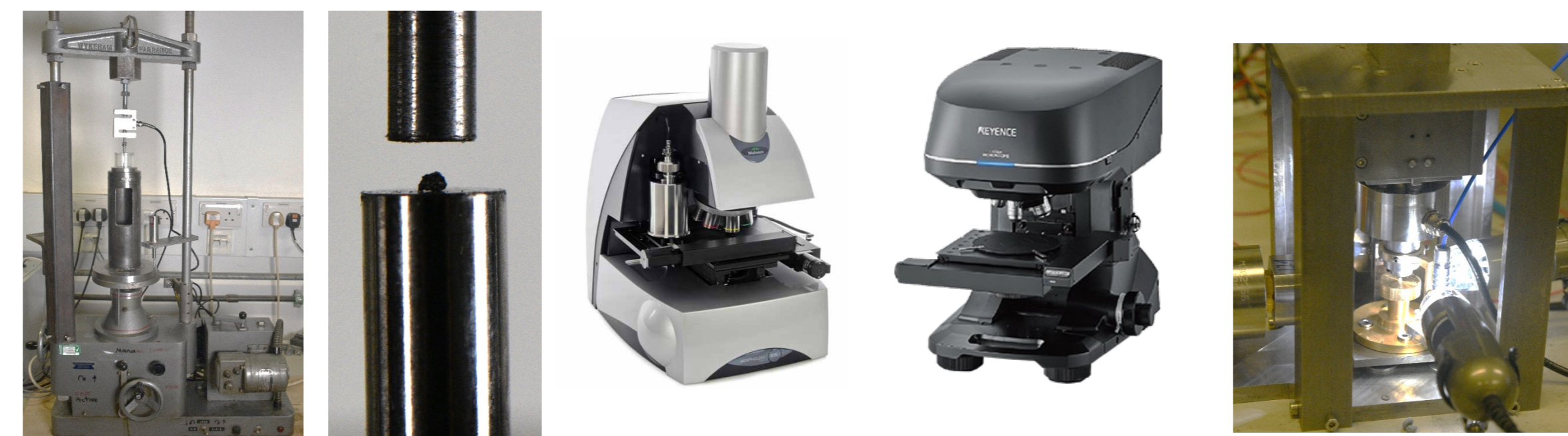
Figure 4. (left) Whole setup of loading frame, (right) particle in between the two platens.
