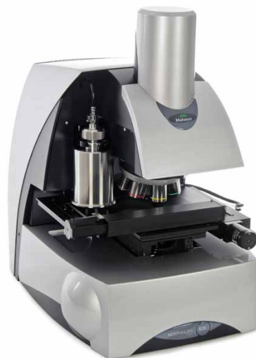
Figure 10. Malvern Morphologi machine, equipped with 5 magnification levels and scans particles down to 0.5 microns (Malvern, 2021)
