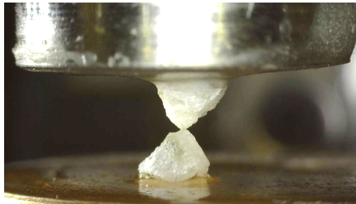
Figure 36. Image taken of Anorthosite vs Anorthosite inside the interparticle apparatus, particles used are around 1mm in diameter.
