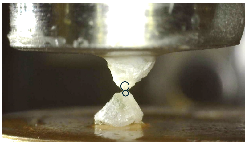
Figure 15. Image of two anorthosite particles with peaks in contact inside the Interparticle apparatus
