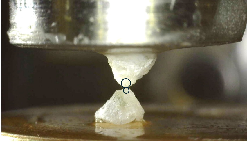
Figure 5. Image of circle used to collect radius of circle that circumscribes the arc of the contact point of the particle
