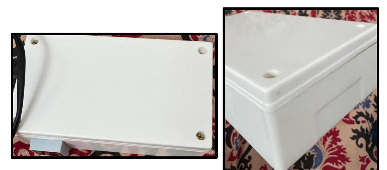
Figure 5. Secure sealing of the voltage logger box
