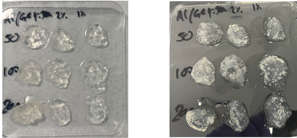
Figure 8. Hydrogels prepared with different concentration of alginate(4%, 2% and 1%)-gelatin(2%) and CaCl_2 (200, 100 and 50 mM)
