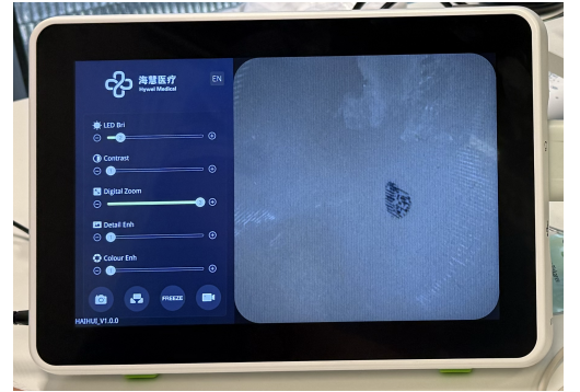
Figure 5: Test setup: the nephroscope inserted through a PVA sheath simulating one of the three percutaneous access points, with a supervisor present throughout testing (left), and a marked calyx as viewed on the monitor, used as the reachability criterion (right).
