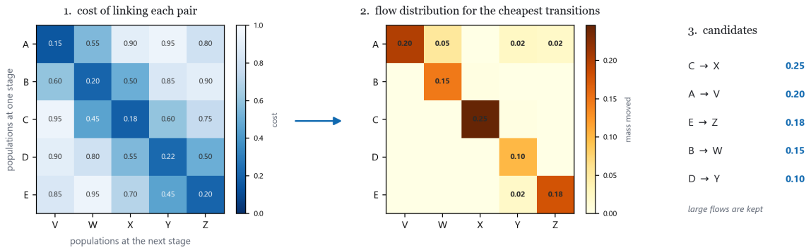
Figure 4. How optimal transport chooses candidates: An example with five populations per stage. The flows in the second matrix are the resulting optimal transport solution based on the first.
