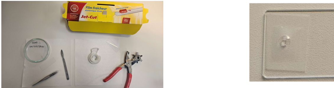
Figure 11: The PDMS/PVC stamp used for pick-up and transfer. Left: the tools and materials used to assemble the stamp (glass slide, PDMS cube, PVC film, scalpel, tweezers and a hole punch). Right: close-up of the finished stamp, showing the PDMS square exposed through the hole cut in the PVC film [9].
