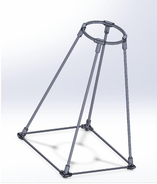
Figure 3: CAD design of the drone stand (left) and the final physical assembly (right).
