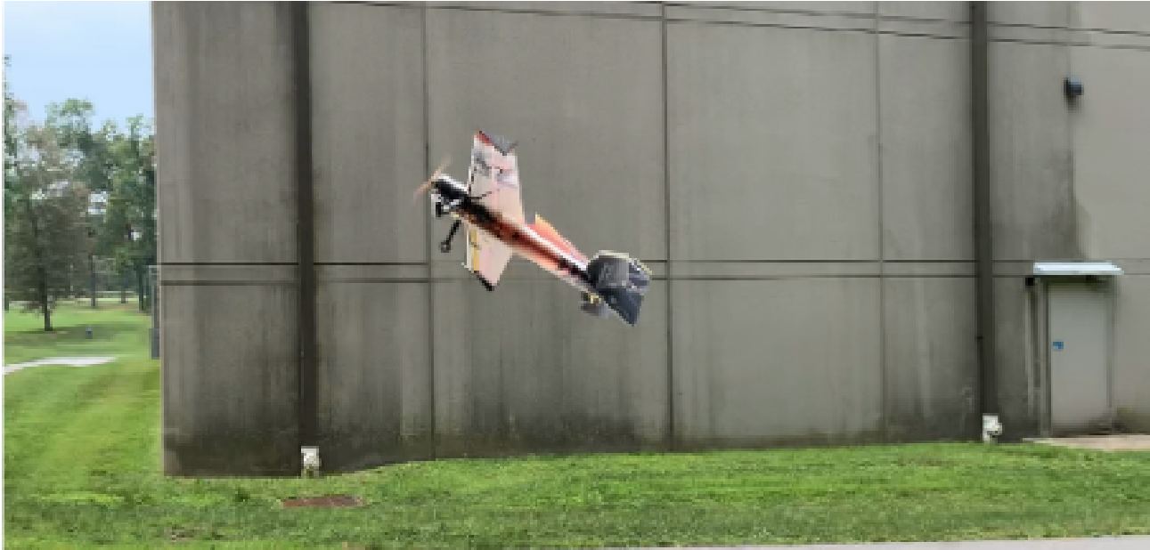
Fixed-wing aircraft, 100 g, 65 cm span
