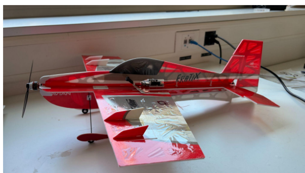
Figure 1. The F3P aircraft used in this project: a 100 g fixed-wing aeroplane with a 65 cm span, flown indoors.
