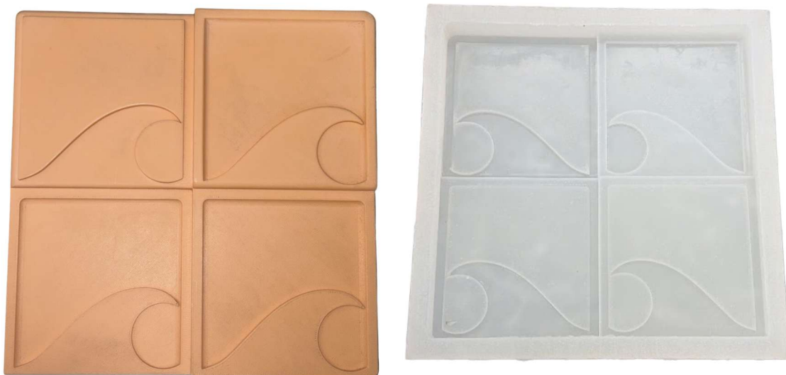
Figure B1. 3D-printed master architectural panel pattern and silicone mould used for casting.
