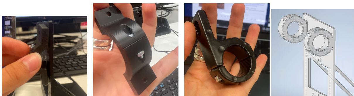
Figure 8. The bracket went through several iterations before the nut-inside design, which fits a 3D-printed part and leaves room for the clamp arm.
